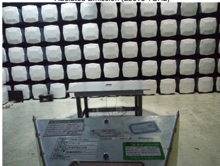
Radiated Emission (above 1GHz)
