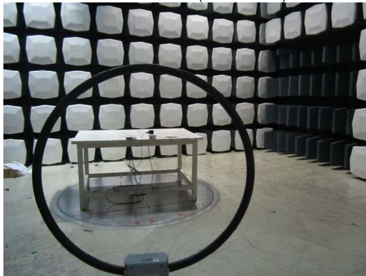
Radiated Emission (Below 30MHz)
