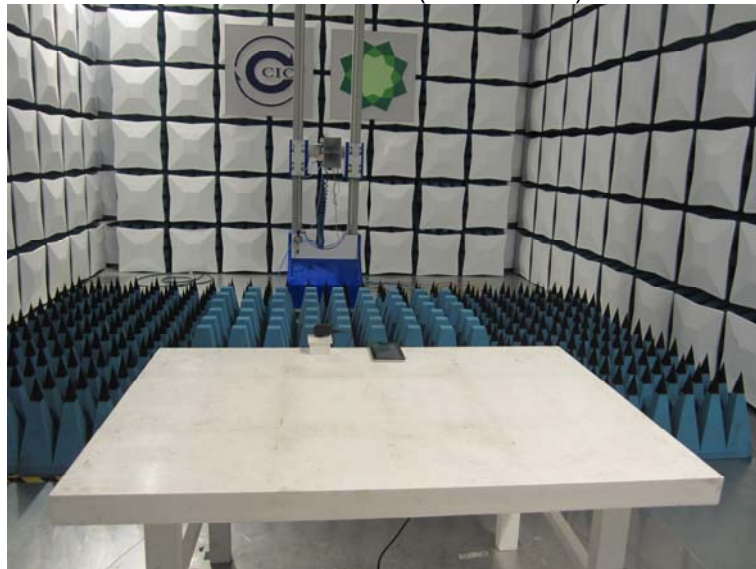
Radiated Emission (Below 30MHz)
