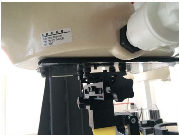
0mm Body-worn Rear Side Setup Photo
