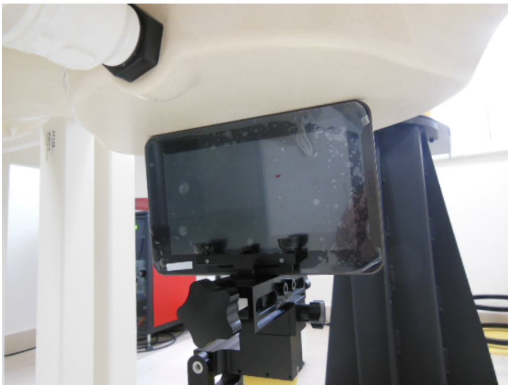
0mm Body-worn Right Side Setup Photo
