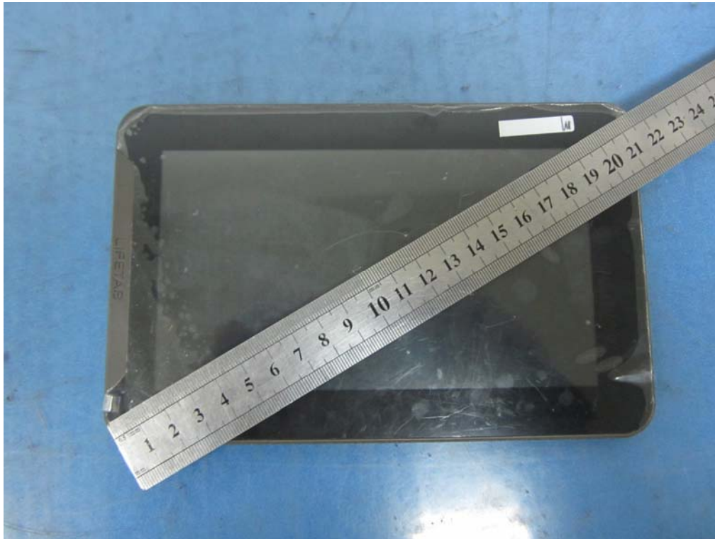
Figure 1: The diagonal dimension of the DUT
