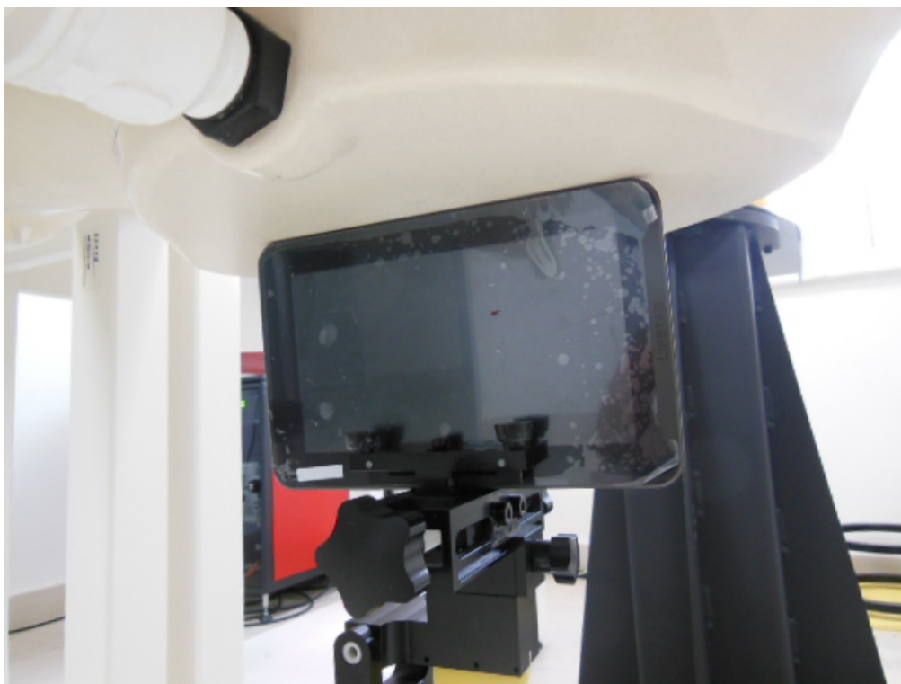
0mm Body-worn Right Side Setup Photo
