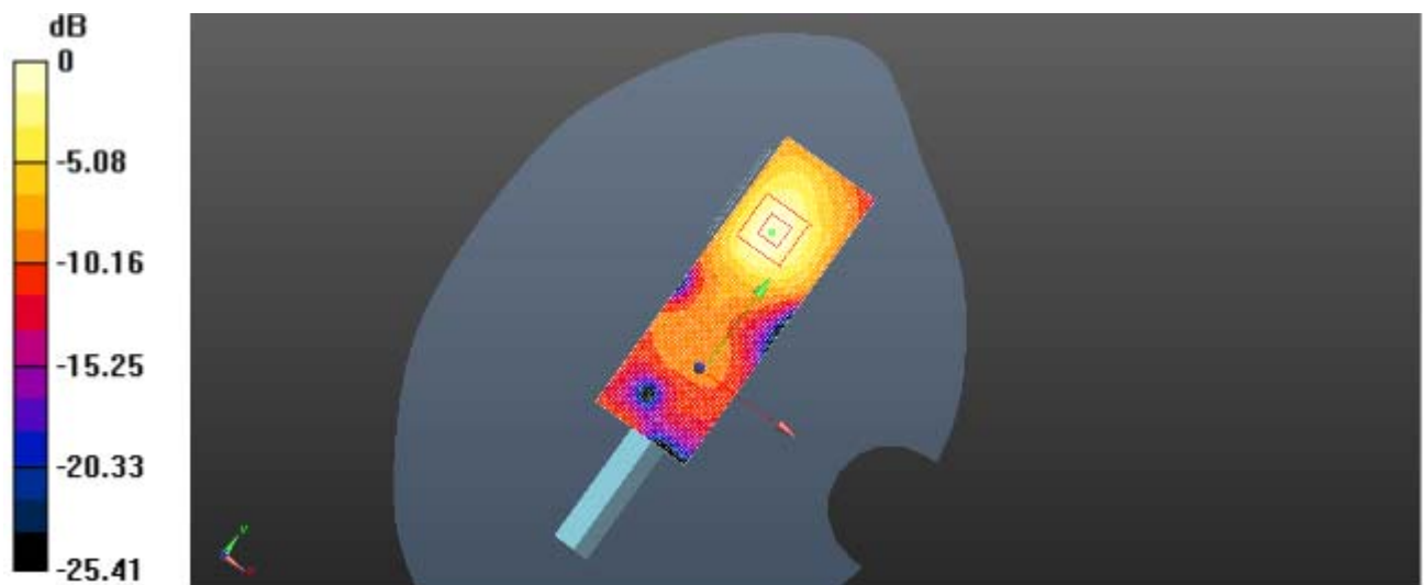
Plot 7: Front Side (WLAN2450-Middle Channel-Channel 6-2437MHz(1Mbps))
