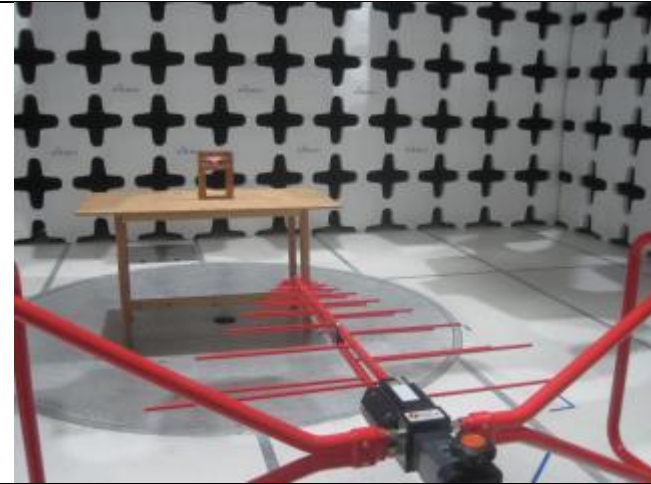
Radiated Emission Test setup (<1GHz) – Front View
