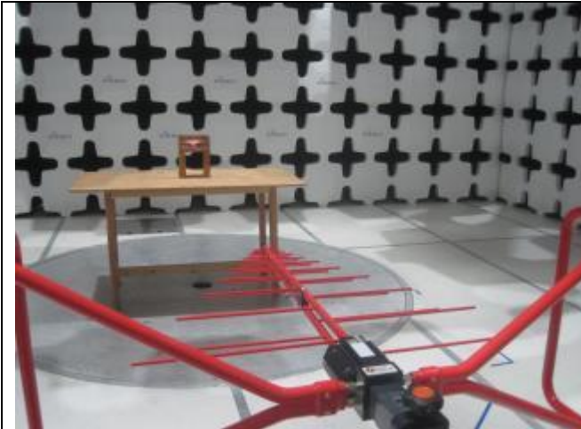
Radiated Emission Test setup (<1GHz) – Front View
