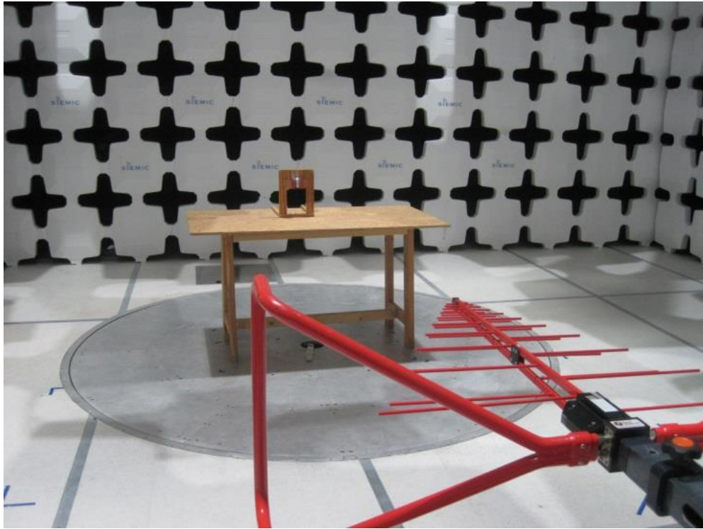
Radiated Emission Test setup (<1GHz) - Front
