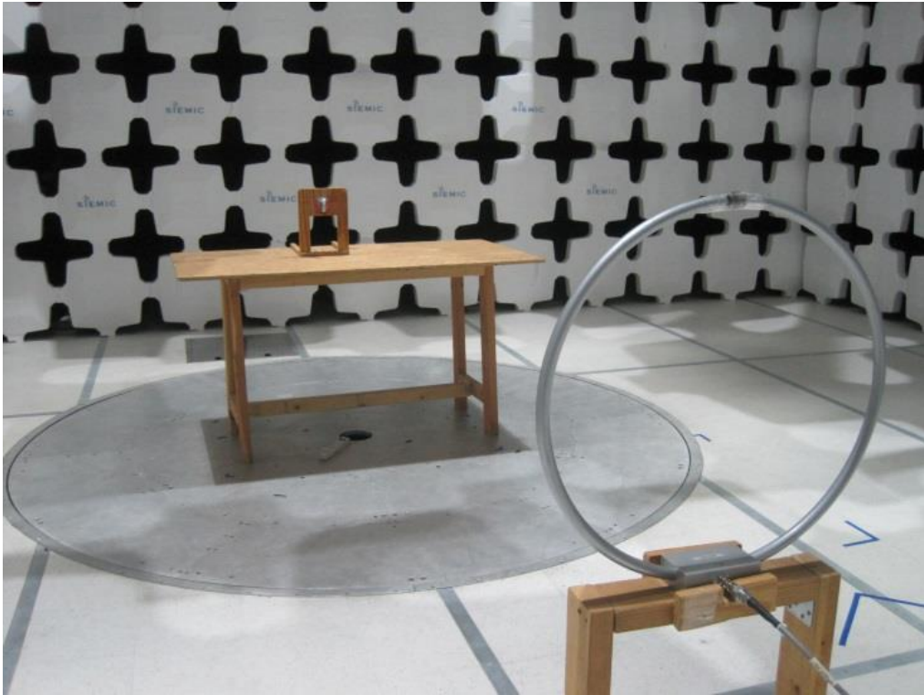
Radiated Emission Test setup (<30MHz) - Front
