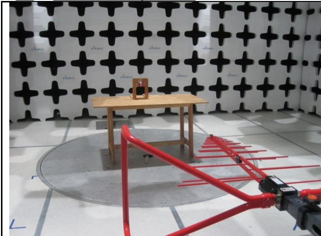
Radiated Emission Test setup (<1GHz) - Front
