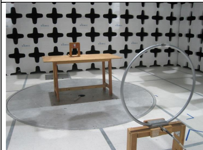
Radiated Emission Test setup (<30MHz) - Front
