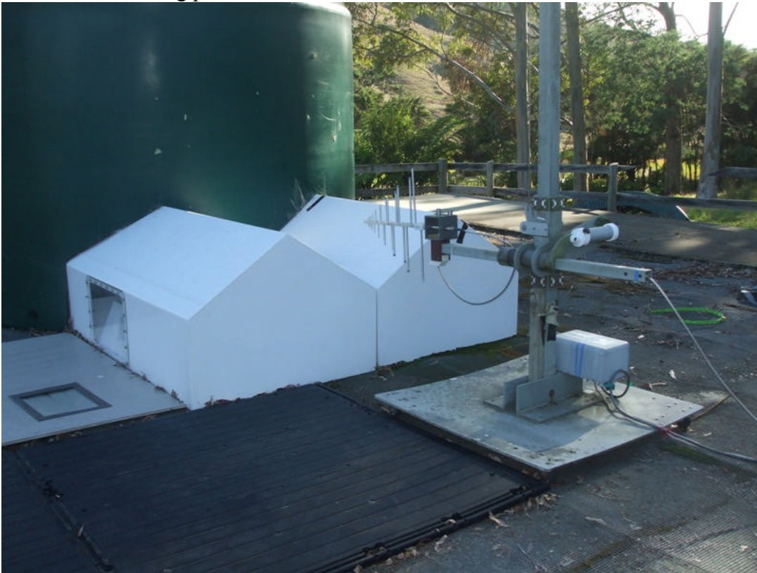
300 – 1000 MHz log periodic antenna
