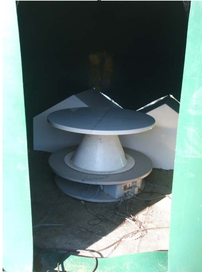
Inside the test enclosure showing the turntable and cone enclosures
