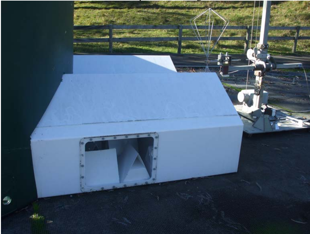
Cone enclosure up close showing the cones
