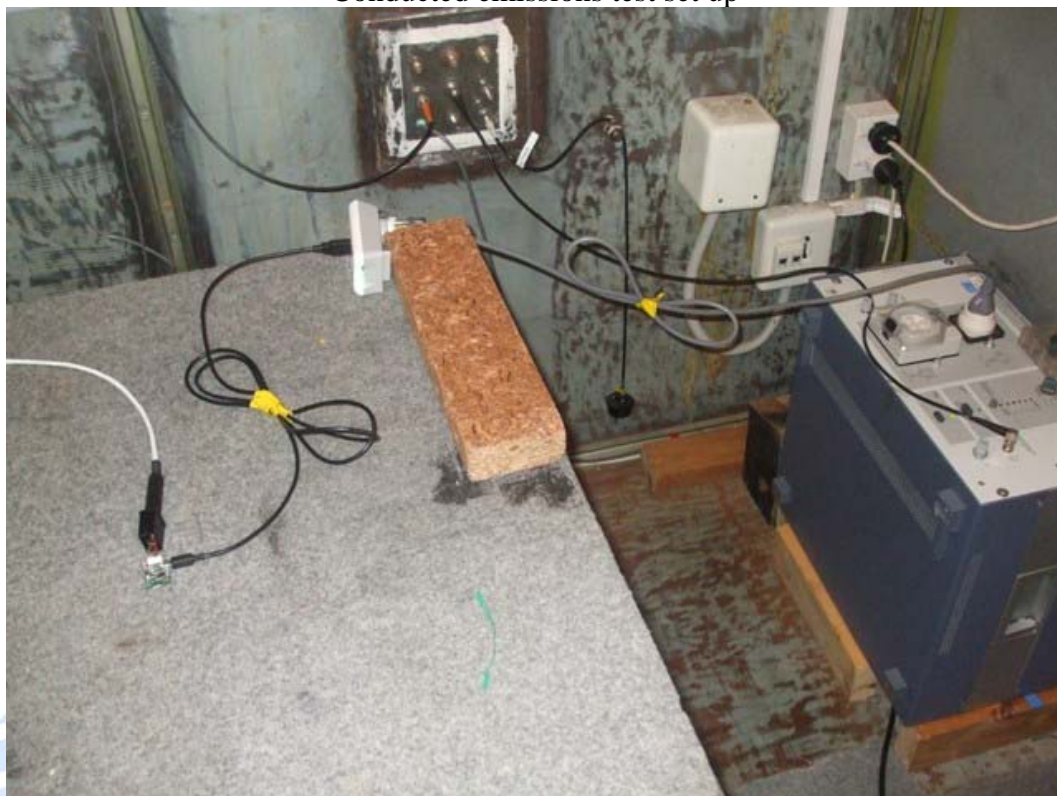
Conducted emissions test set up
