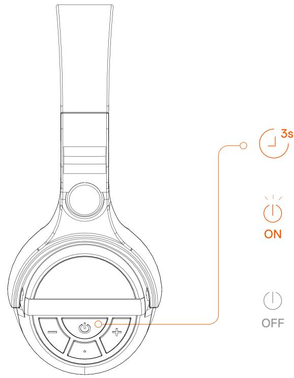
To power on the headset press and hold the power button for at least 3 seconds. The LED indicator will Red.
