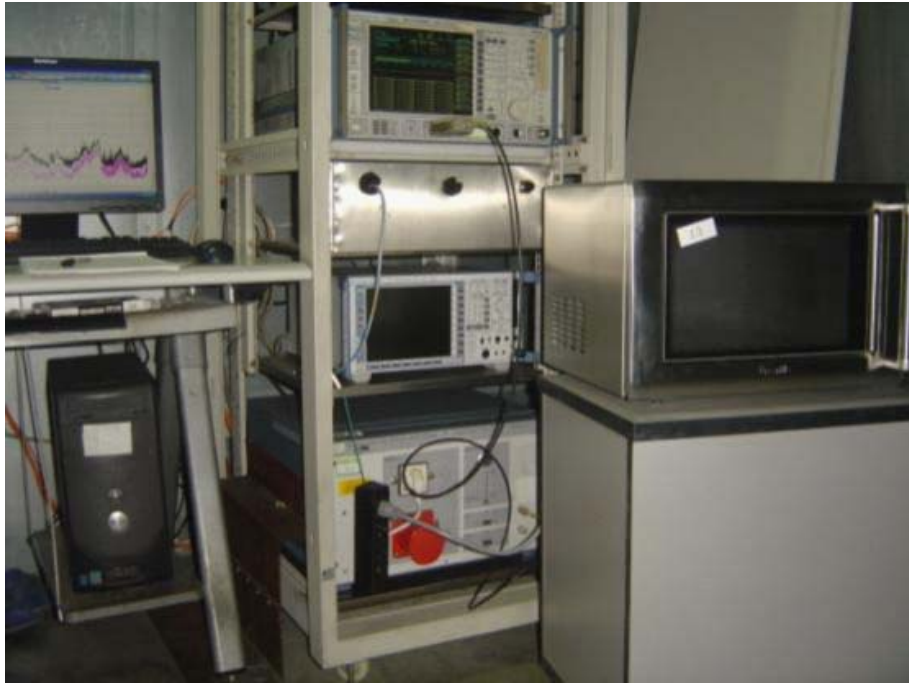
Conducted Emission Test Set-up
