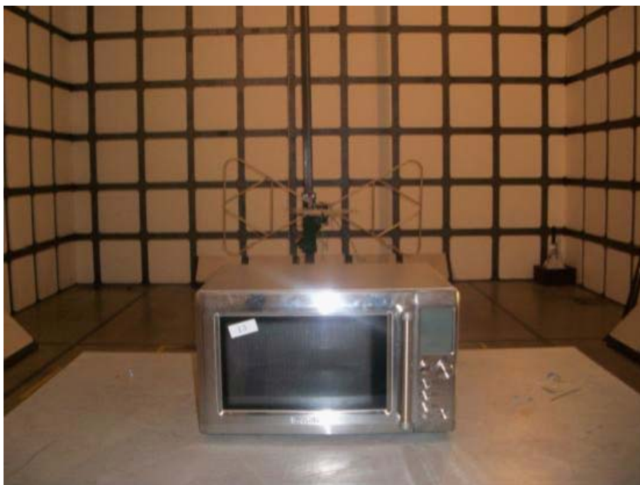
Radiated Emission Test Set-up (30 -1,000MHz)
