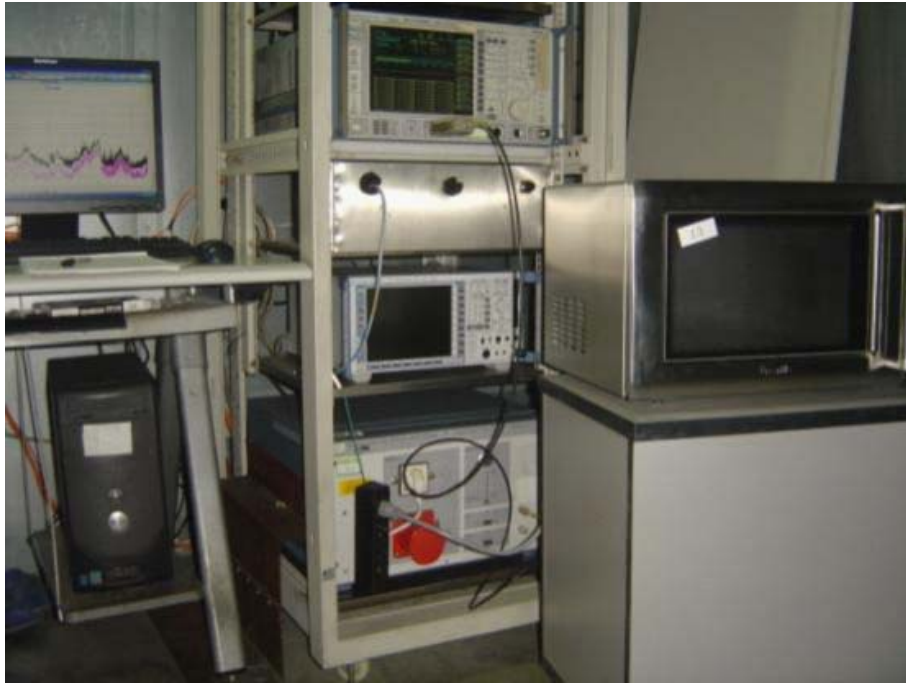
Conducted Emission Test Set-up
