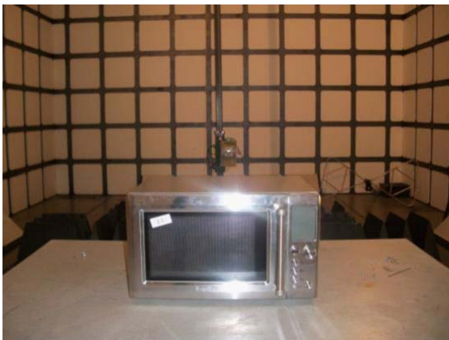
Radiated Emission Test Set-up (1-18GHz)
