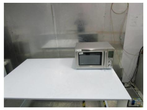
1.2 Radiated Emissions (30MHz-1GHz) Test Setup
