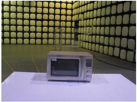
Radiated Emissions (Magnetic field Strength)(9kHz-30MHz)
