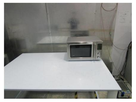
1.2 Radiated Emissions (30MHz-1GHz) Test Setup
