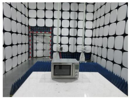
1.4 Radiated Emissions (Magnetic field Strength) (9kHz-30MHz) Test Setup
