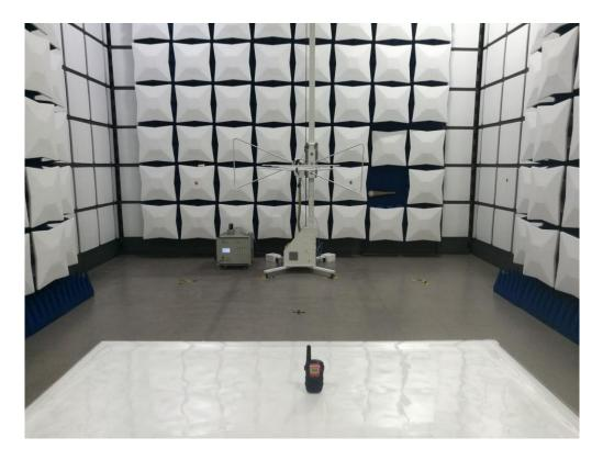
RADIATED EMISSION ABOVE 1G TEST SETUP
