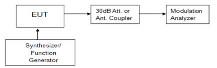
Figure 1: Modulation characteristic measurement configuration
