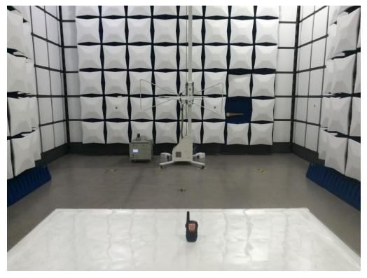
RADIATED EMISSION ABOVE 1G TEST SETUP
