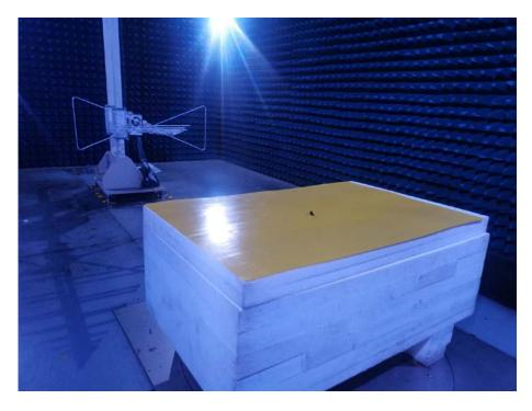
Photo of Radiated Emission Measurement Above 1GHz
