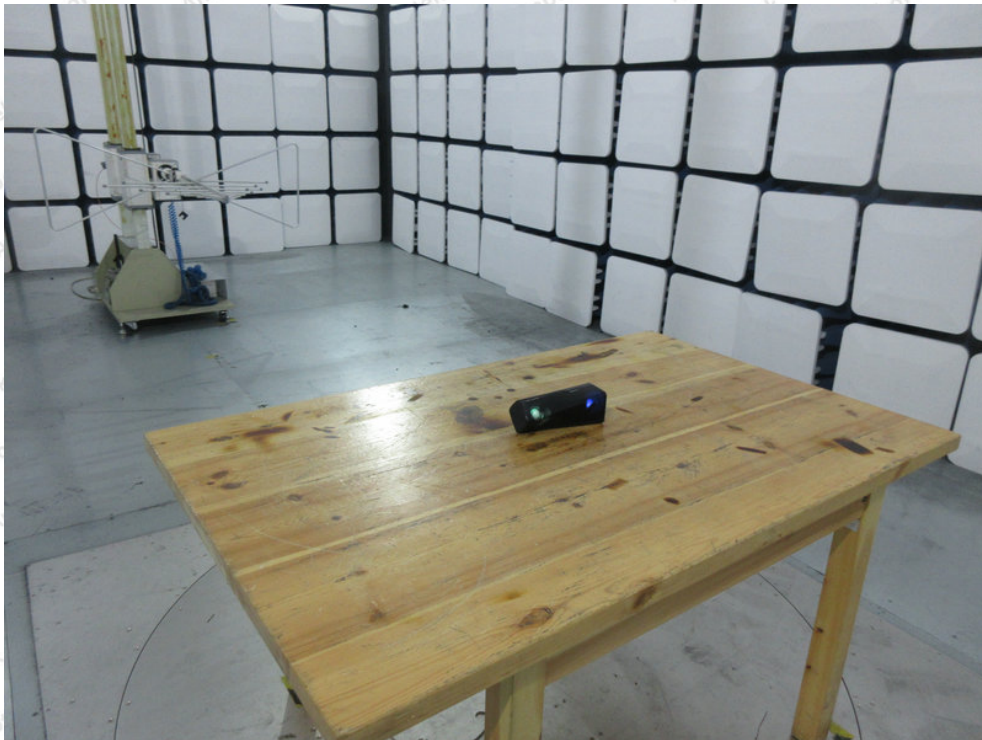
Photo of Radiation Emission Test
