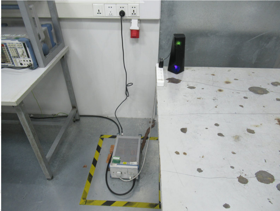
Photo of Conducted Emission Measurement
