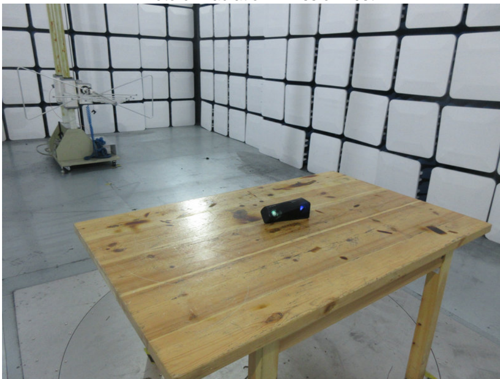
Photo of Radiation Emission Test
