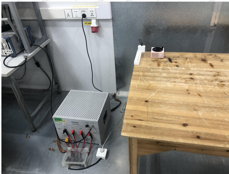
Photo of Conducted Emission Measurement
