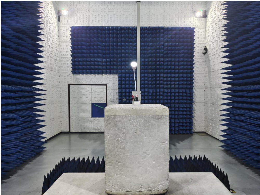
RADIATED EMISSION TEST SETUP ABOVE 1GHz
