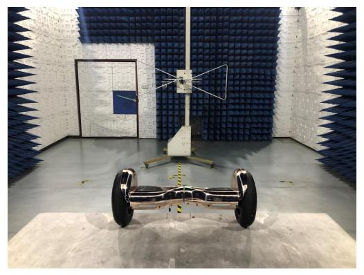
RADIATED EMISSION TEST SETUP ABOVE 1GHz
