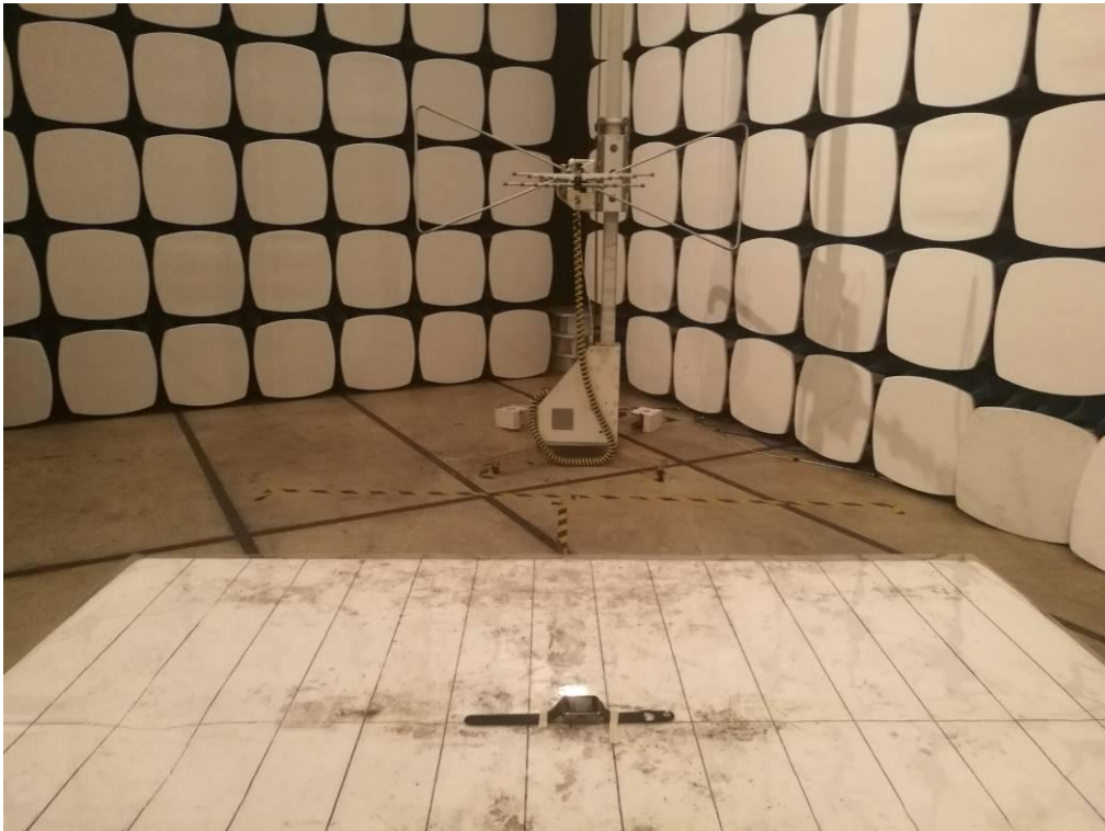
FCC RADIATED EMISSION TEST SETUP
