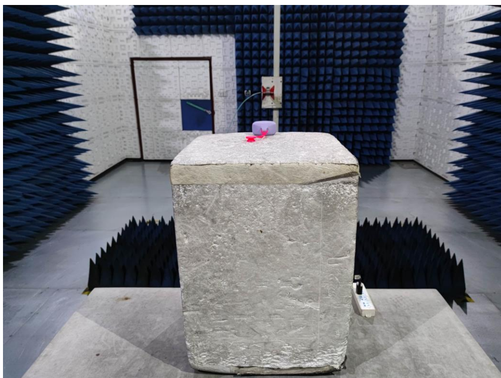
RADIATED EMISSION TEST SETUP ABOVE 1GHz
