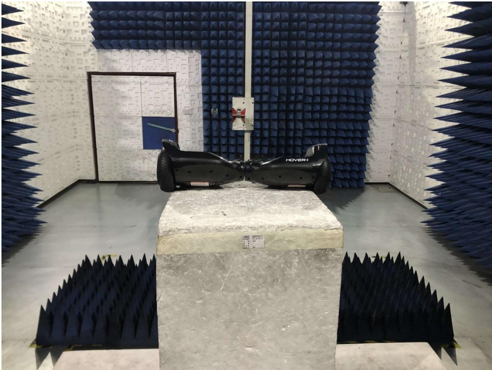
RADIATED EMISSION TEST SETUP ABOVE 1GHZ
