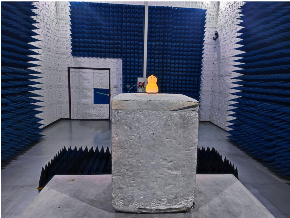
RADIATED EMISSION TEST SETUP ABOVE 1GHz
