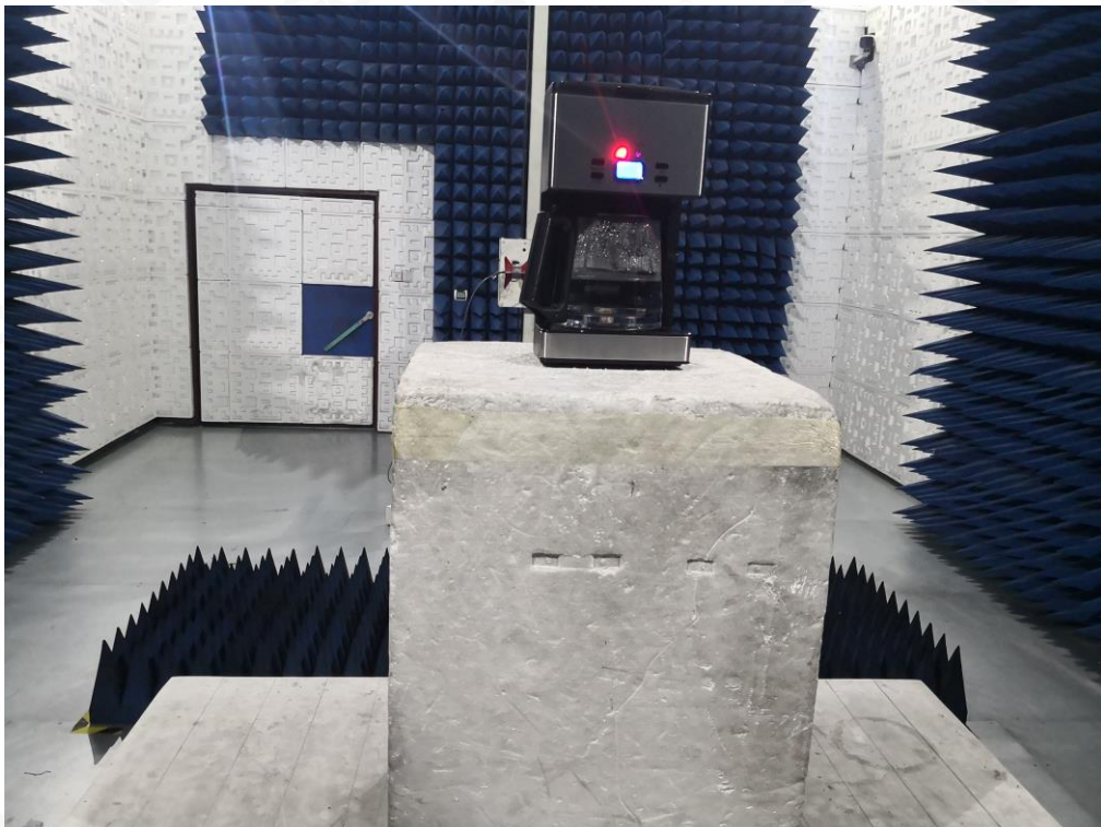
FCC RADIATED EMISSION TEST SETUP ABOVE 1GHZ
