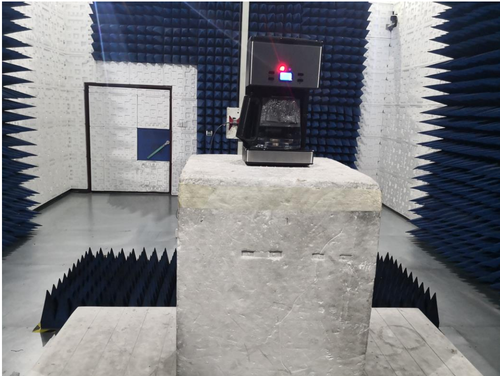
FCC RADIATED EMISSION TEST SETUP ABOVE 1GHZ
