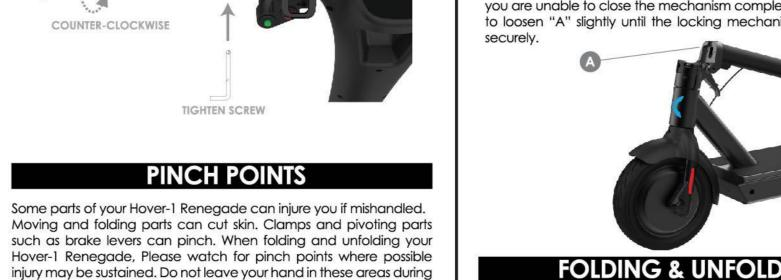
FOLDING & UNFOLDING FOLDING & UNFOLDING YOUR RENEGADE SCOOTER. To unfold your Renegade, press down on the folding clip and pull the steering column up. Raise the safety lock up and push it into place to secure the steering column. You will hear a "click", indicating the steering column is locked. Ensure the steering column is secured in
