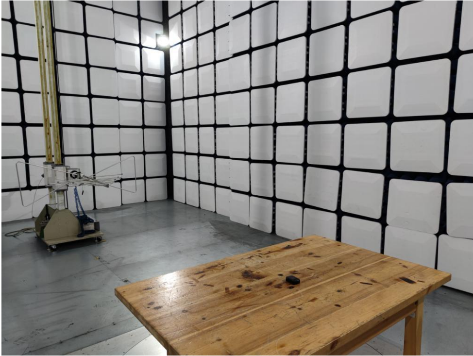
Photo of Radiation Emission Test
