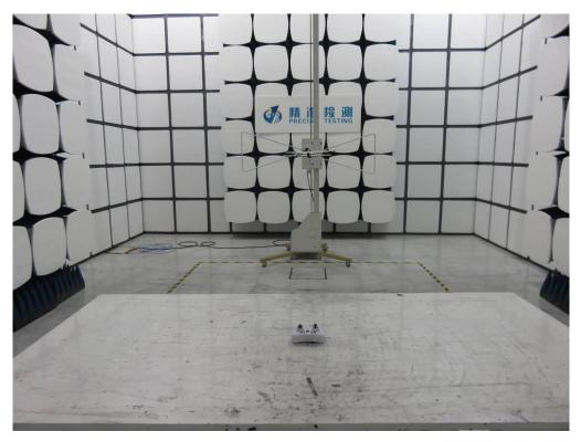
RADIATED EMISSION TEST SETUP ABOVE 1GHz
