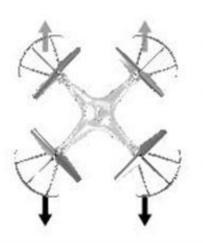
In the case that the aircraft is hovering in the air and the aircraft still fly forward or backward, this time you can correct it by pushing the trimmer upward or downward.
