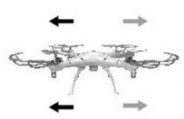
In the case that the aircraft is hovering in the air and the aircraft still fly to the left or to the right, you can correct it by pushing the trimmer to the right or to the left.
