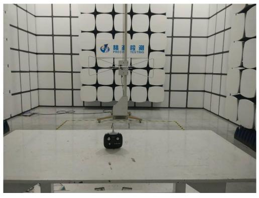
RADIATED EMISSION TEST SETUP ABOVE 1GHz
