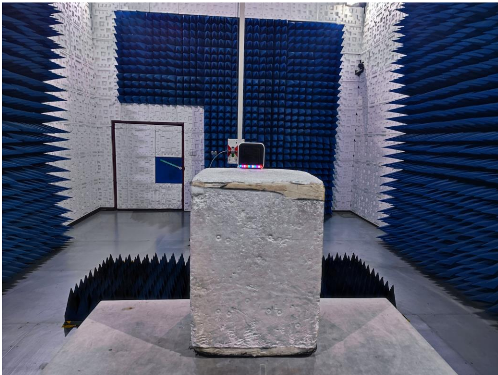
RADIATED EMISSION TEST SETUP ABOVE 1GHZ
