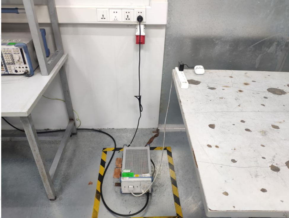
Photo of Conducted Emission Measurement
