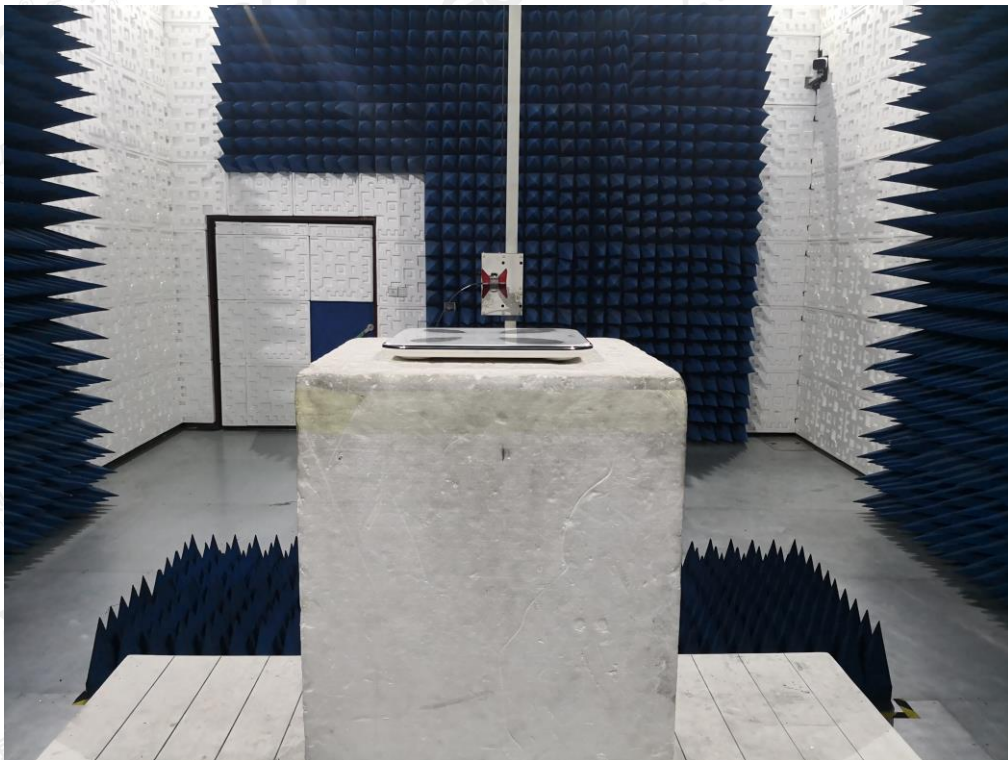
FCC RADIATED EMISSION TEST SETUP ABOVE 1GHZ
