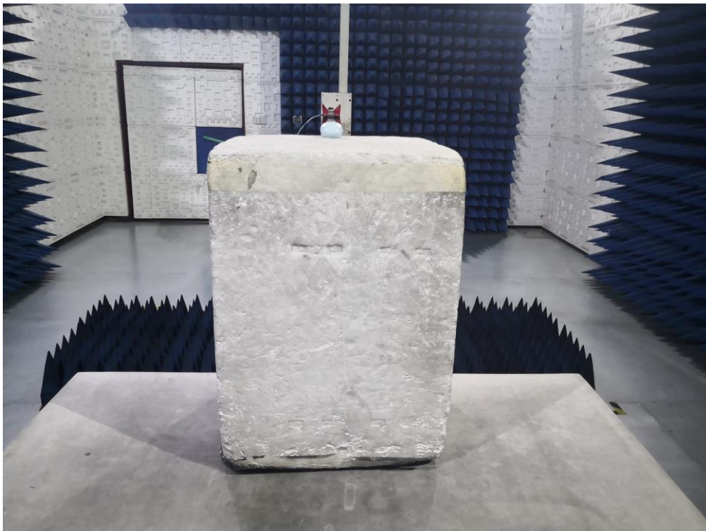
RADIATED EMISSION TEST SETUP ABOVE 1GHz
