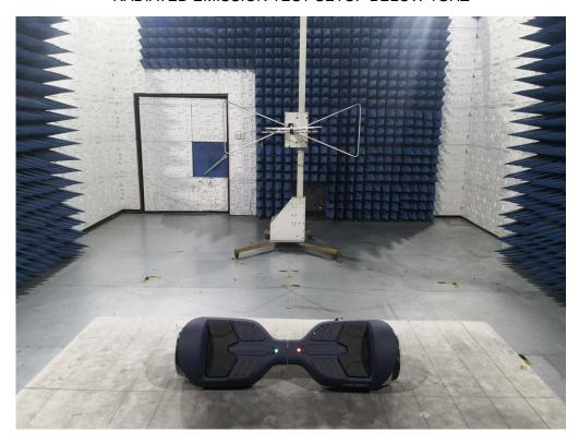
RADIATED EMISSION TEST SETUP ABOVE 1GHZ
