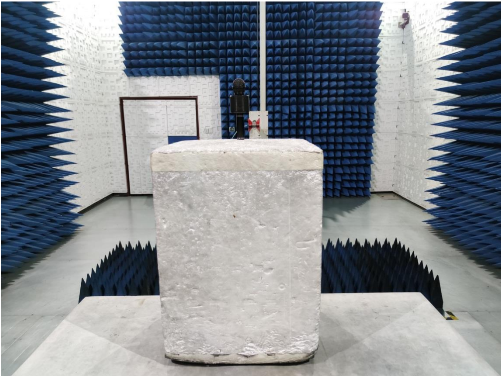
RADIATED EMISSION TEST SETUP ABOVE 1GHz
