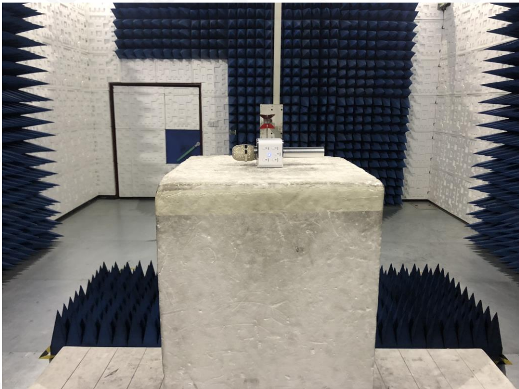
RADIATED EMISSION TEST SETUP ABOVE 1GHZ
