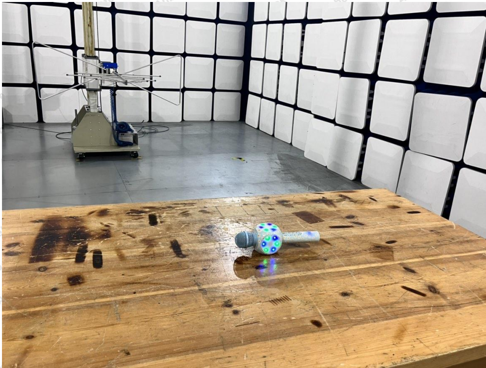
Photo of Radiation Emission Test
