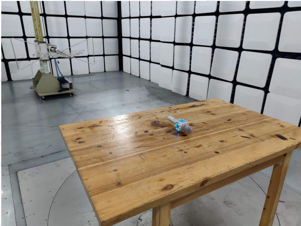
Photo of Radiation Emission Test
