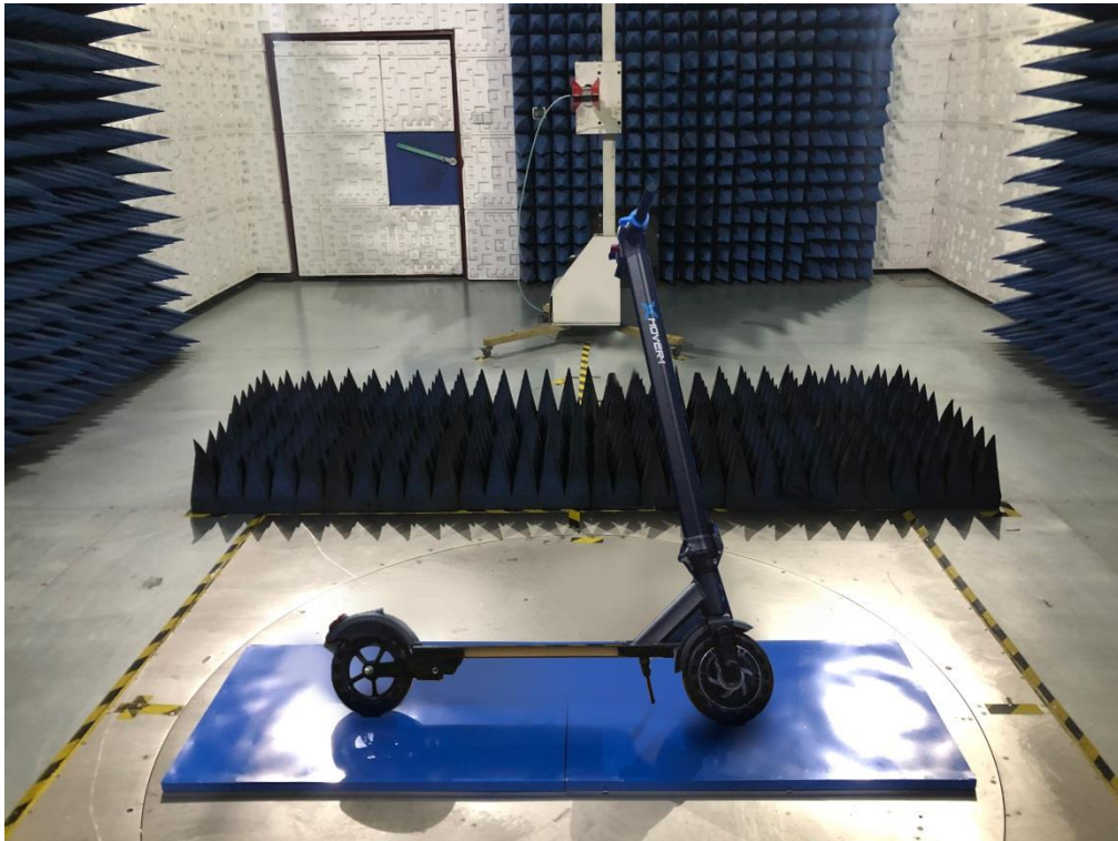
RADIATED EMISSION TEST SETUP ABOVE 1GHz
