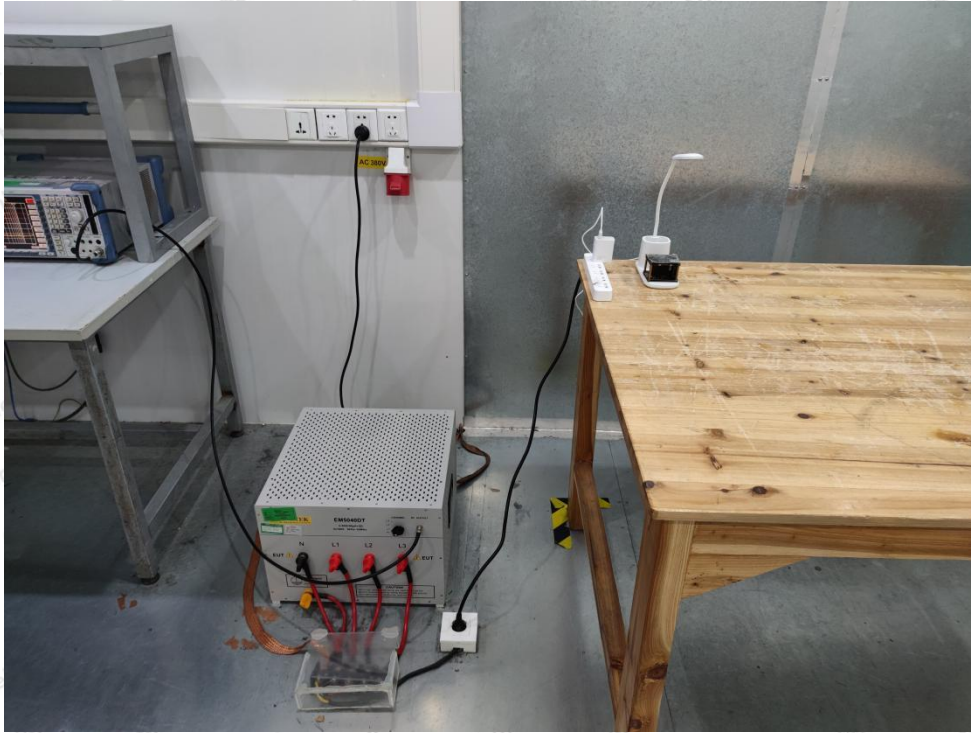
Photo of Conducted Emission Measurement
