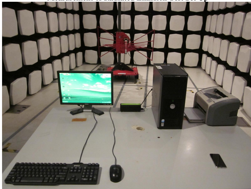
Measurement of Radiated Emission Test Set Up
