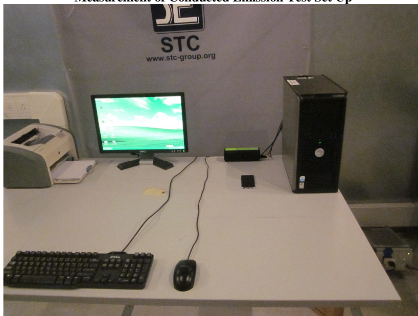
Measurement of Conducted Emission Test Set Up
