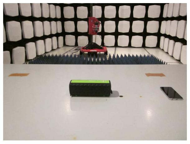
**MEASUREMENT OF CONDUCTED EMISSION TEST SET UP**
