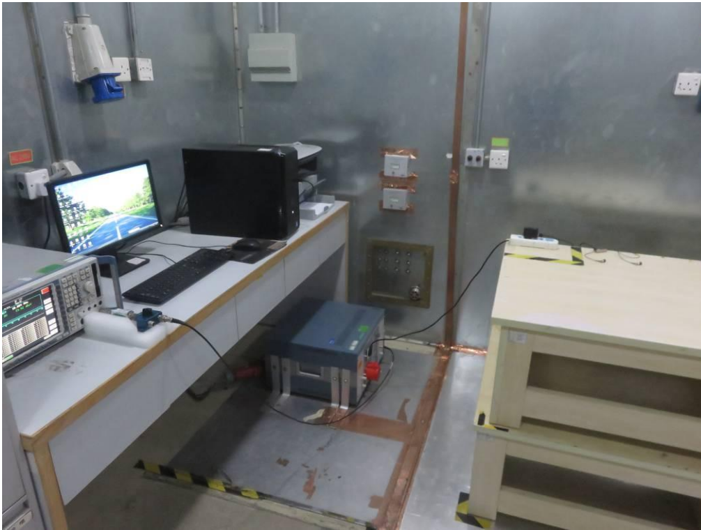
FCC RADIATED EMISSION TEST SETUP
